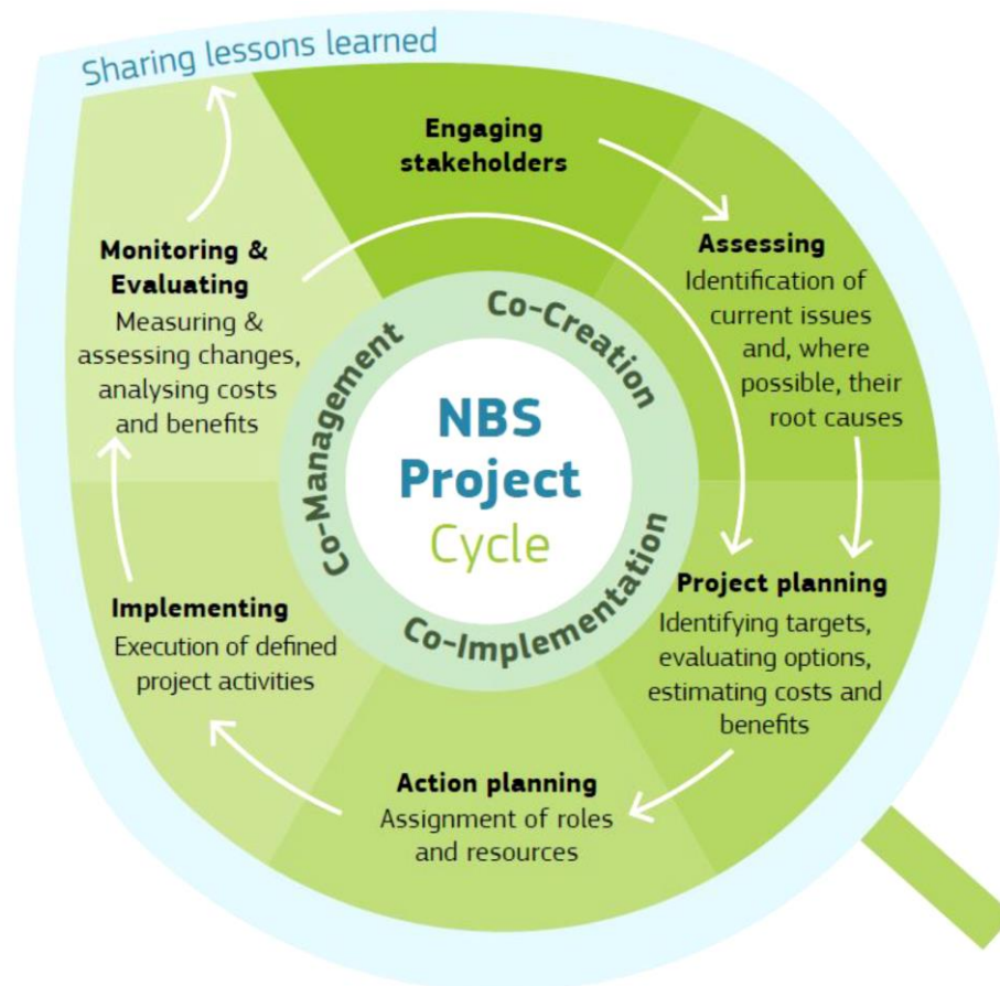
Fig. 3.10 A schematic diagram showing the full project life cycle of NBS such as monitoring and evaluation, cost benefit analysis (adapted from Kumar et al. , 2020)
